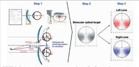
FIGURE 1 Beginning with individual eye parameters, SynchronEyes Technology™ creates a binocular optical system in which optical quality is balanced at homologous points on each lens.
